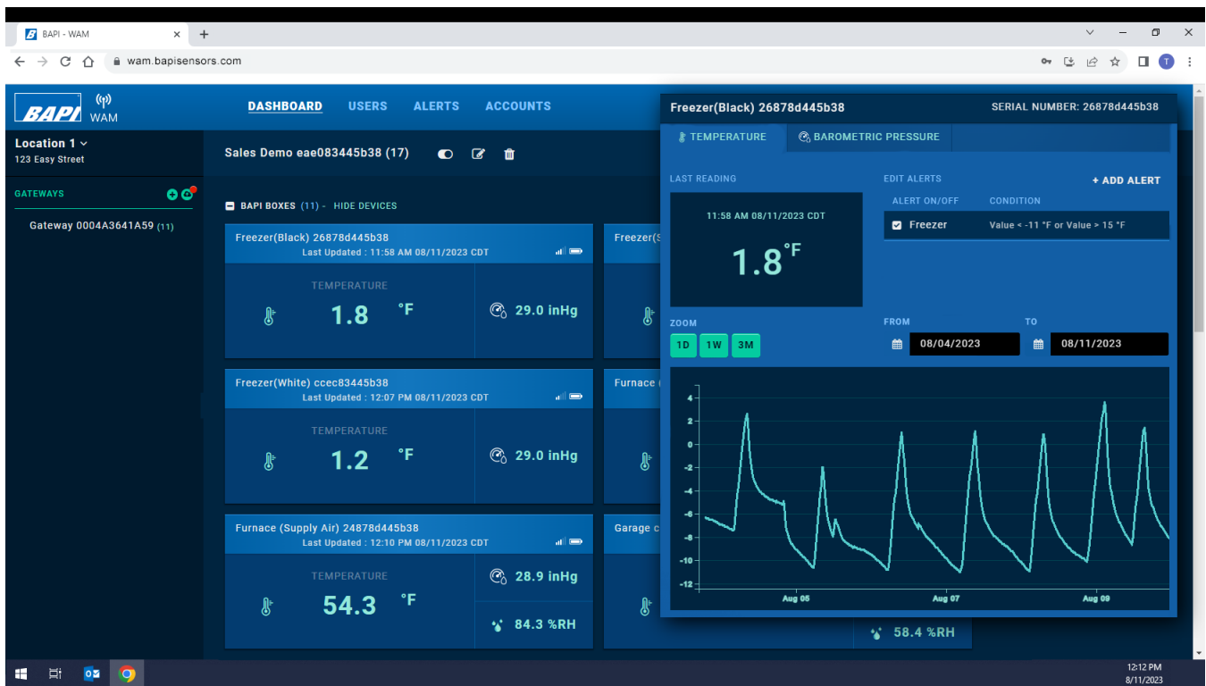
Fig. 12: BAPI WAM Website “Dashboard” screen showing multiple sensors and a sensor trend.
